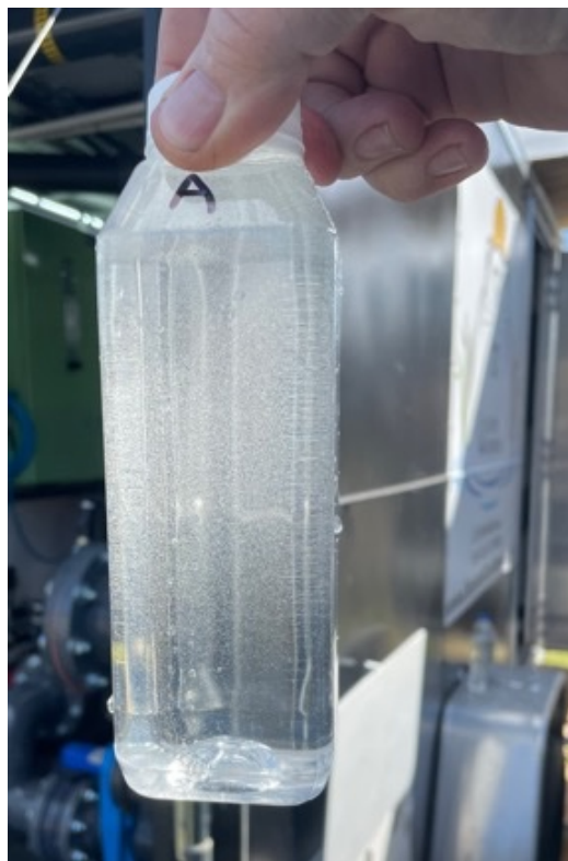
Figure 13. Treated water is shown saturated with oxygen-rich macrobubbles.
