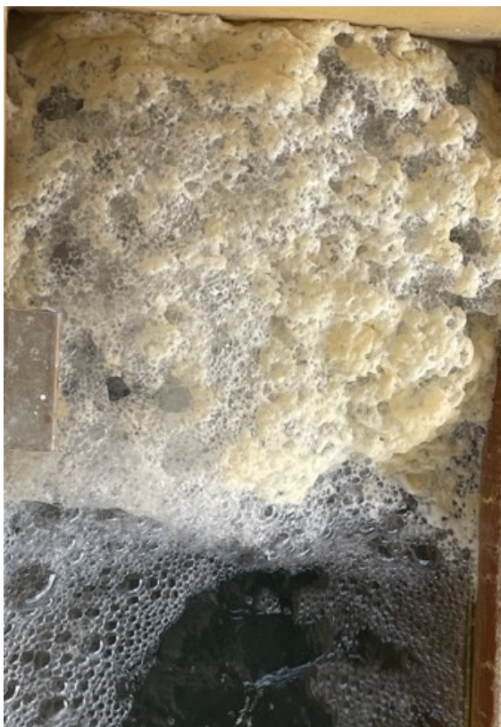
Figure 10. Scum collecting at the top of the collection tanks, which demonstrates oxidation of iron and hardness precipitation.
